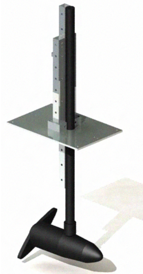
Figure 3: Rendered SolidWorks drawing of the machined aluminum motor mount with the motor and attached U-Channel in place
