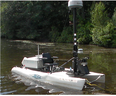
Fig. 2. Olin Intelligent Vehicles Lab ASV Medea. Medea is based on a 12-foot Hobie catamaran and has a fold-down mast for an 18 inch radome.
