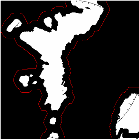
Fig. 3. Radar image after undergoing morphological operations to isolate the path around the shore. The white objects are obstacles as detected by radar, and the red path represents the allowed path around the shore.
