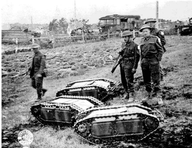
Figure 3. The WWII German Goliath explosive charge carriers are an early example of teleoperated robots. Image courtesy of Military History Monthly magazine.*
