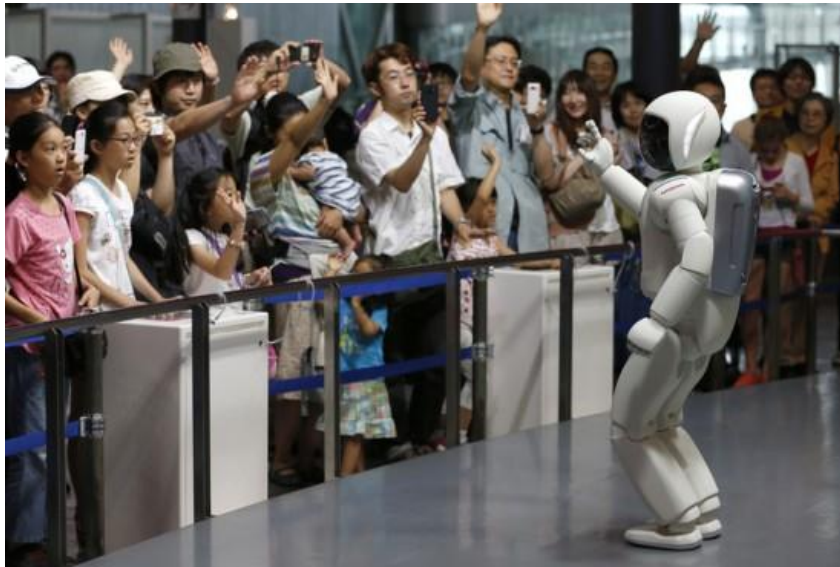
Figure 4. Honda’s Asimo , Tokyo’s Mirakan Science Museum’s new tour guide, as it was unveiled to the public in July. Asimo cannot differentiate between someone asking a question or raising their smartphone in the air to take a picture—and can only be asked pre-determined questions through a touchscreen interface. Image courtesy of Japan Daily Press.§
