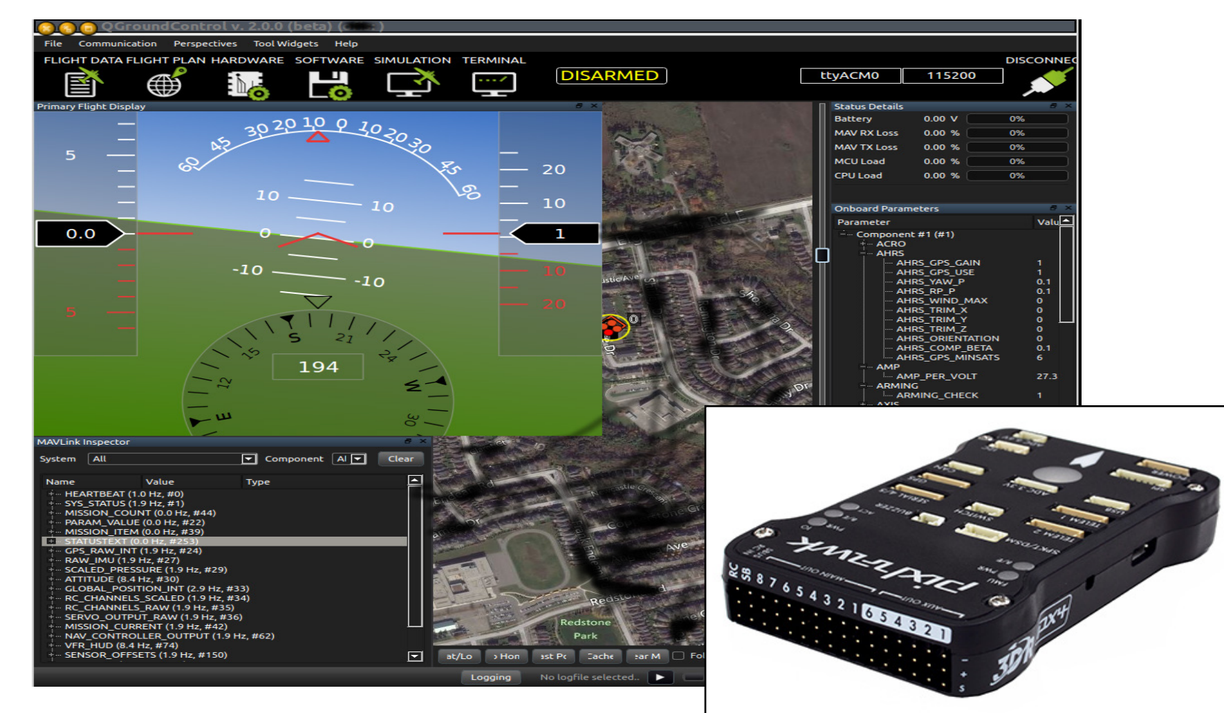
The Pixhawk in conjunction with QGroundControl is an open-source autopilot system. We will use this system as a communications layer between our code and this autopilot system.
